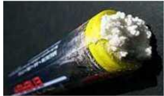
Fig.1 A Leaking Electrochemical Battery
