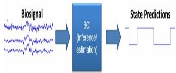
Figure 4 BCI Block dig.
