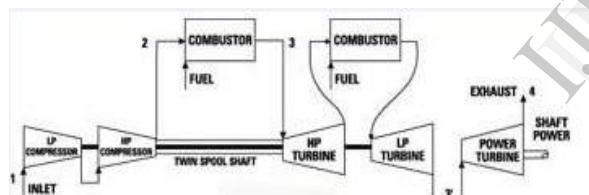
Reheating requires extra combustors which obviously increase cost of equipment and also fuel to reheat the gas. But, reheating is properly utilised when it is used in combustion with regeneration and also inter-cooling.
