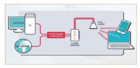
Li-Fi operates on simple binary encoding using variations in light intensity. The system comprises three core components:
