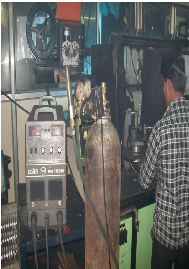
Figure 2 MIG Welding setup
