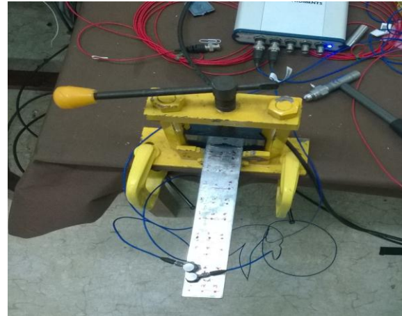
Fig 6 Test setup for OMA.
