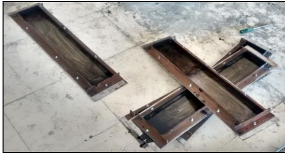
Figure I: Flexure Test moulds
