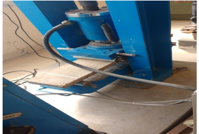
Figure III: Flexural test on specimen
