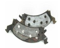
The heavier the vehicle, the more brake dust you'll see on the front wheels versus the rear. In most cases a simple steel spring is riveted to the brake pad backing plate to serve this purpose. When the friction material wears to the point that replacement is necessary, the spring will contact the rotor, emitting a high-pitched squeal.
