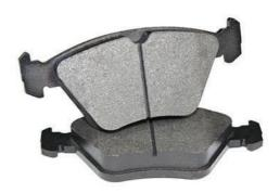
Brake pads are a component of disk brakes used in automotive and other applications. Brake pads are steel backing plates with friction material bound to the surface that faces the disk brake rotor. Two brake pads are contained in the brake calliper with their friction surfaces facing the rotor. When the brakes are hydraulically applied, the calliper clamps or squeezes the two pads together into the spinning rotor to slow/stop the vehicle. Then providing the friction that stops the vehicle.
