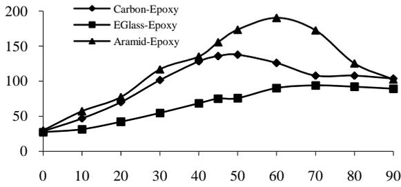
Fig 8. Bending stress vs winding angle
