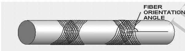
Figure 12 - Fiber orientation for  $45^{\circ}$  and  $-45^{\circ}$
