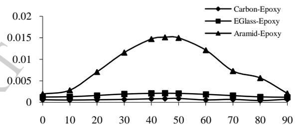
Fig 5. Angle of twist vs winding angle
