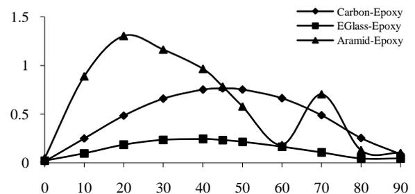
Fig 6. Radial deformation vs winding angle
