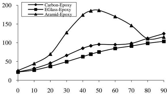
Fig 9. Shear stress vs winding angle
