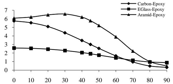
Fig 3. Axial deformation vs winding angle
