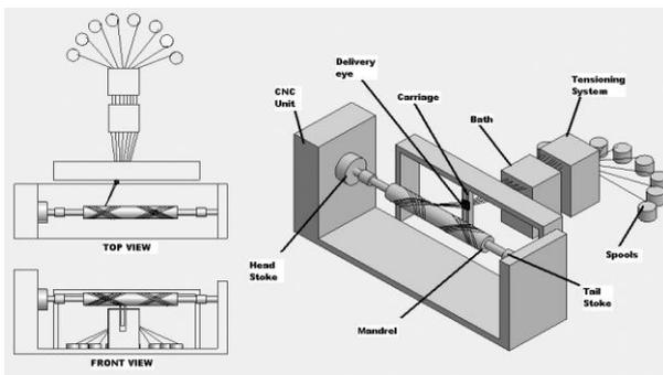
Figure 11 – Schematic View of a Filament Winding Machine
