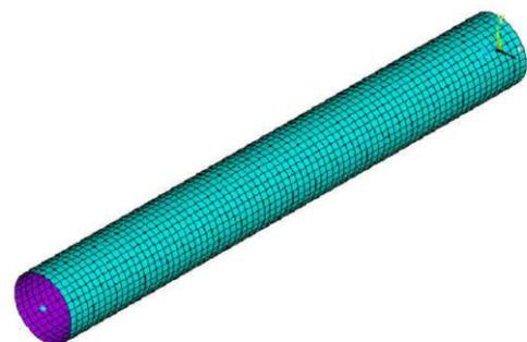
Fig 1. Finite element model of composite tube
