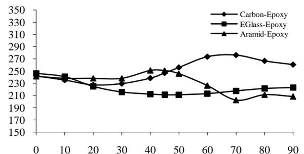
Fig 7. Normal stress vs winding angle
