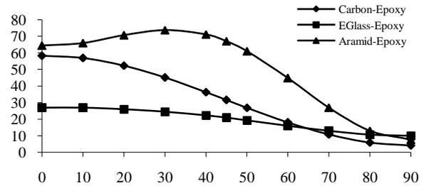
Fig 4. Lateral deformation vs winding angle
