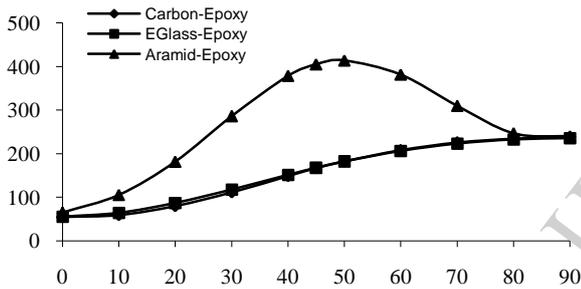
Fig 10. Hoop stress vs winding angle
