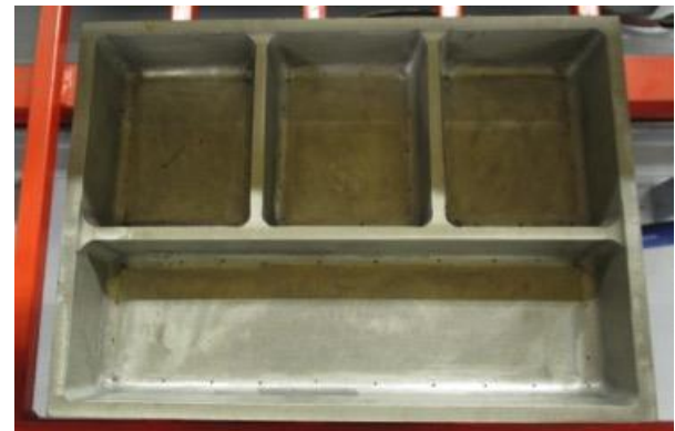
Figure 5. Aluminum mold with vacuum holes
