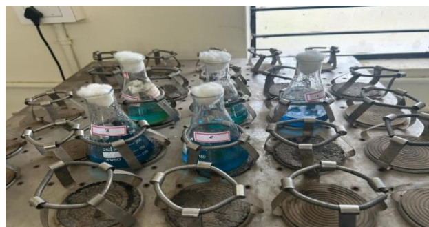
Fig 3 Agitation of the samples in the shaker at 50 RPM
