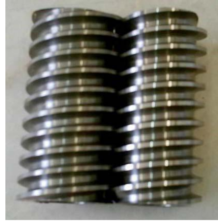
Figure 7 The final modules of the self-wipe screw prepared with Lathe machine by using Special cutting tool shape
