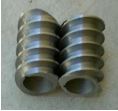
Figure 6 Screws prepared by lathe machine-by using of mould
