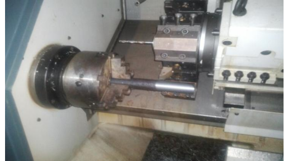
Fig 1.1. Machining of EN 8 steel in CNC machine
