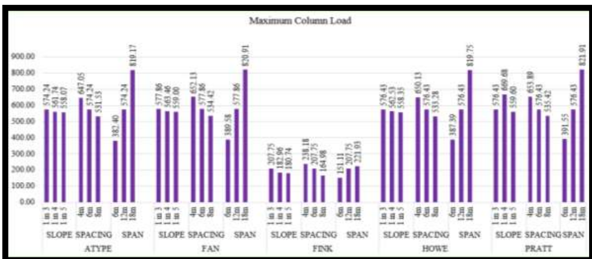
Fig. 10: Graph showing the maximum column load for all the truss models
