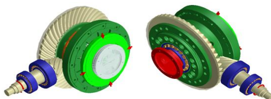
Fig. 3.6 Differential lock layout
