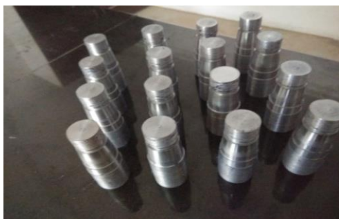
FIGURE3.3.TEST SPECIMEN AFTER MACHINING
