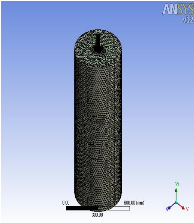
Fig 2: Meshing modal of tank
