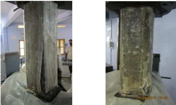
Fig.13 Failure modes of Unconfined specimens
