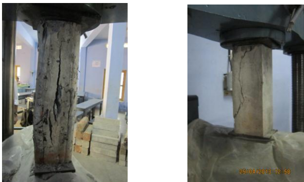
Fig.13 Failure modes of Unconfined specimens
