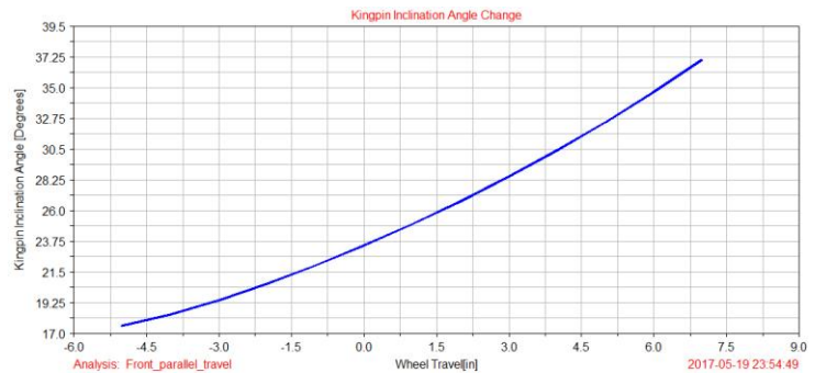
Fig. 12. Kingpin Inclination angle VS Wheel travel.
