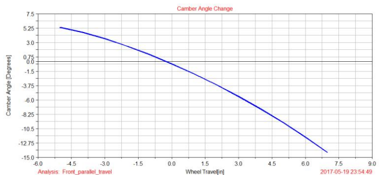
Fig. 4. Camber angle VS Wheel travel.
