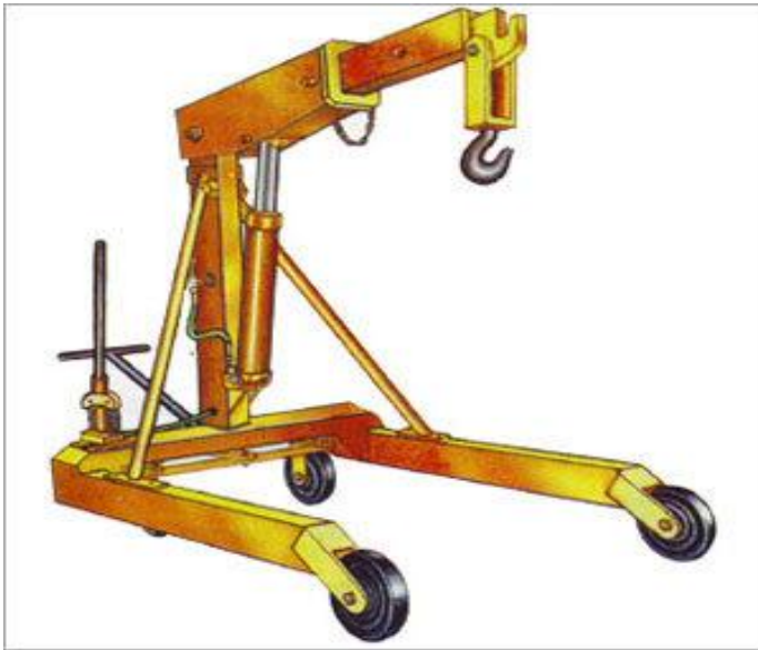
Figure (1) Computer Model for Hydraulic Floor Crane
