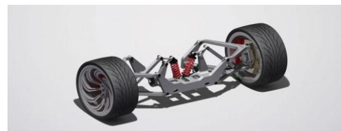
Figure 1 : Double wishbone suspension system
