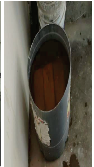
Fig. 4.3 Curing of bricks for water absorption test
