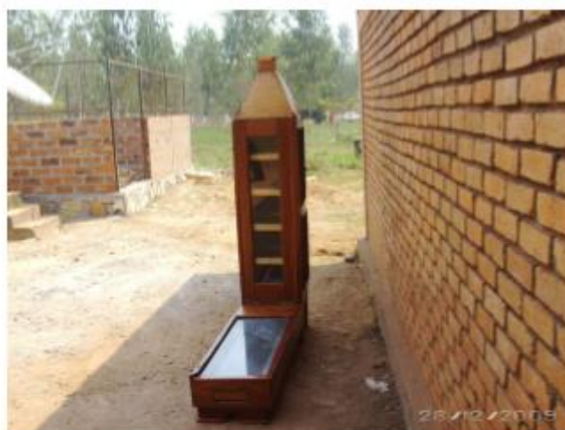
Figure 1: photograph of the foldable and portable double-glazed dryer
