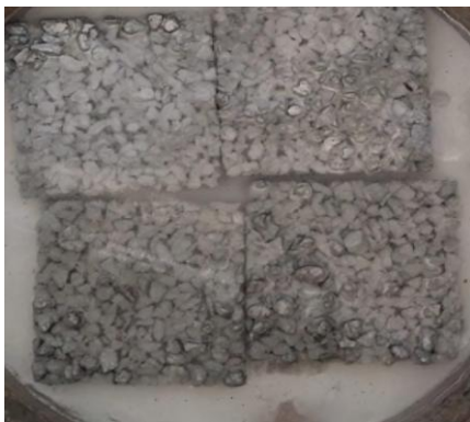
Fig. 1 Submerged bio-concrete specimens with white CaCO 3 deposition indicating active biomineralization
