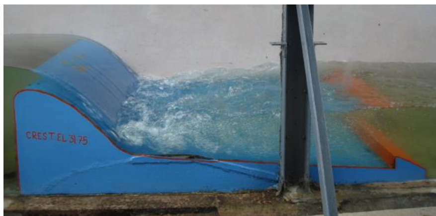
Fig 3. Performance of stilling basin while passing 15700 \text{ m}^3/\text{s} (Sloping apron)
