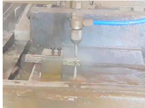
Fig. 3: - Experimental set-up for AWJ cutting.
