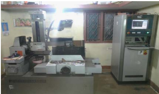
Figure 2: Wire Electrical Discharge Machining Setup
