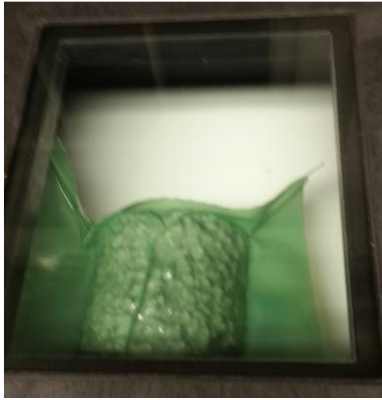
Fig. 4. A sealed pervious concrete sample placed in Corelok
