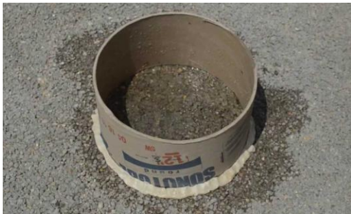
Fig. 6. Single-ring infiltrometer (ASTM C1701)
