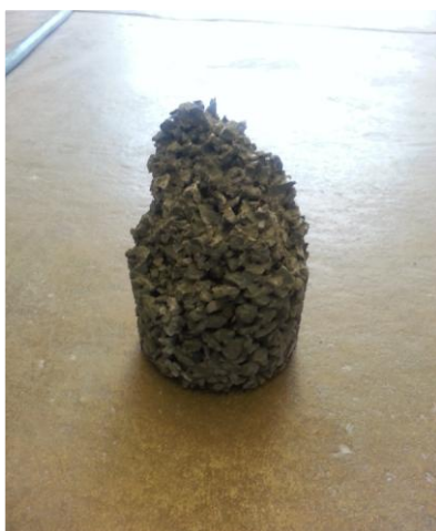
Fig. 2. A sample of failed pervious concrete
