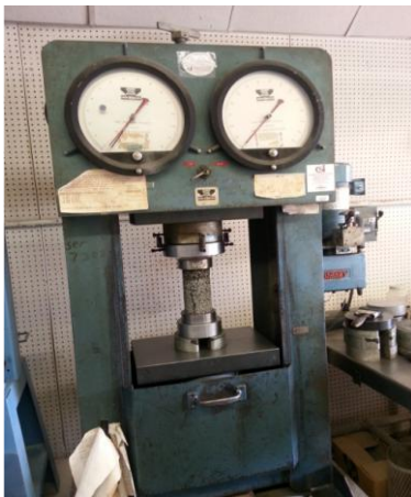
Fig. 1. Concrete cylinder placed in loading frame
