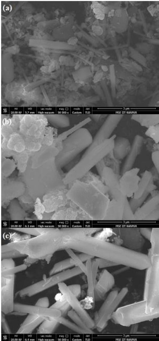
Fig 2: FESEM image of synthesised nanoparticles with 2M KOH as electrolyte at (a) 80V & 30DF, (b) 100V & 25 DF and (c) 120V & 35 DF.
