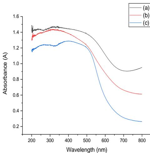
Fig6: UV-Vis absorbance spectra of PbO nanoparticles synthesis with condition: (a) 100 V, 35 DF & 1M, (b) 80 V, 30 DF & 2M and (c) 120 V, 25 DF & 3M of KOH solution.
