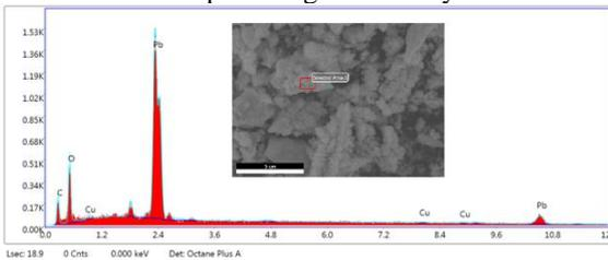
Figure 5: EDX analysis of Cu doped PbO nanoparticles at 120V and 30DF.
