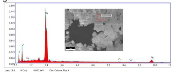
Fig4: EDX analysis of Cu doped PbO nanoparticles at 100V and 35DF.
