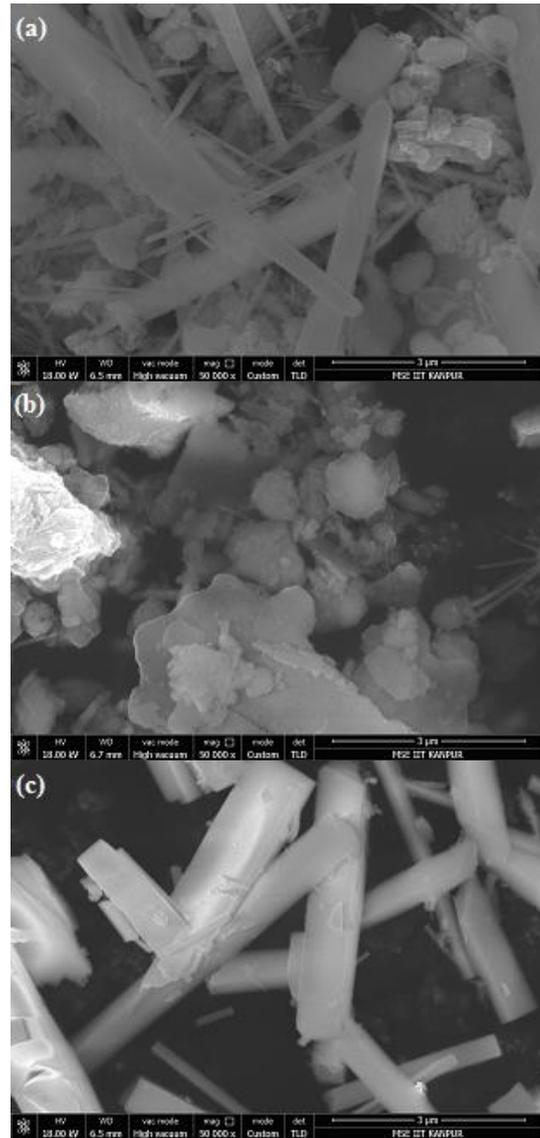
Fig 3: FESEM image of synthesised nanoparticles with 3M KOH as electrolyte at (a) 80V & 35DF, (b) 100V & 30 DF and (c) 120V & 25 DF.
