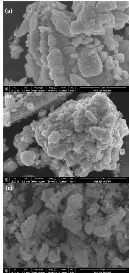
Fig 1: FESEM image of synthesised nanoparticles with 1M KOH as electrolyte at (a) 80V & 25DF, (b) 100V & 35 DF and (c) 120V & 30 DF.
