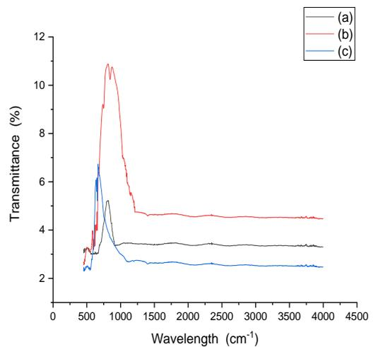
Fig 7: FTIR spectra of PbO nanoparticles synthesis with condition: (a) 80 V, 25 DF & 1M, (b) 100 V, 30 DF & 3M and (c) 120 V, 35 DF & 2M of KOH solution.
