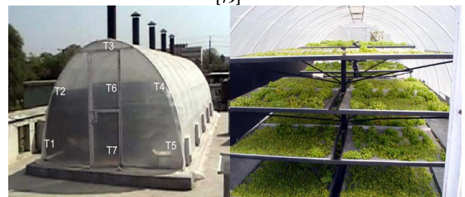
Figure 2.11 Hybrid photovoltaic-thermal (PV/T) integrated greenhouse dryer [79]
