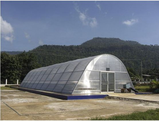
Figure 2.9: solar greenhouse dryer of loading capacity of 1000kg [71]
