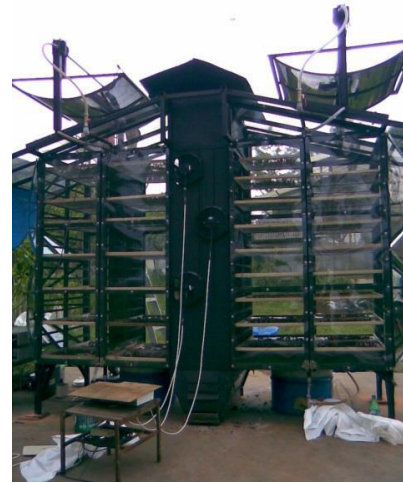
Figure 2.10 Rack type greenhouse solar dryer [73]
