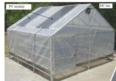
Figure 2.11 Hybrid photovoltaic-thermal (PV/T) integrated greenhouse dryer [79]
