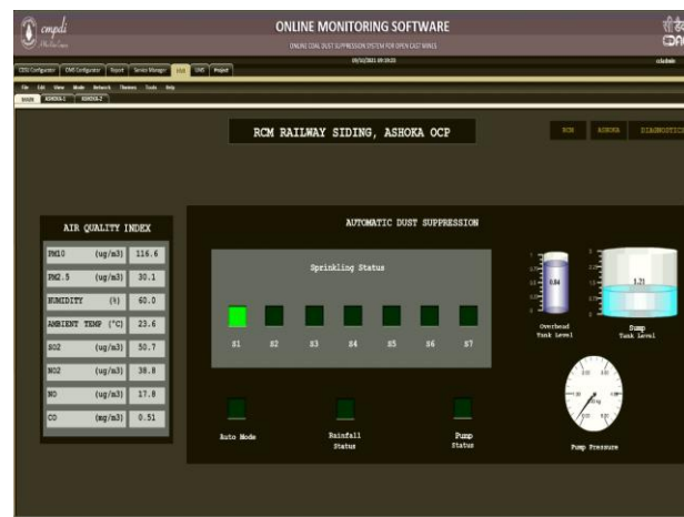
Fig.14. HMI Frame showing sprinkler status
