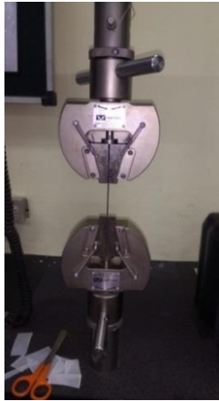
Fig 1: Polyurethane Dumbbell type Specimen & Fixing position in M/s INSTRON
