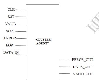
Clusture agent is the combination of receiver, RAM, and packet classification, which forms the clusture module. The cluster module is used as a processing element in a network architecture which is then used with the cell agents or router module to form the overall 4x4 architecture.
