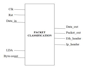
So the Packet classification module is one of the important blocks of the cluster module where the incoming packets are tested and routed to the intended blocks. Since the fault information is available on the cell agent the faulty paths are avoided here. Features of packet classification: LDA pin is used for load axess control.Byte count holds the no of counts or operation done for the i/p data.Ethernet frame header (ETH\_header) is of 26bytes in length and is chosen based on IPV4.
