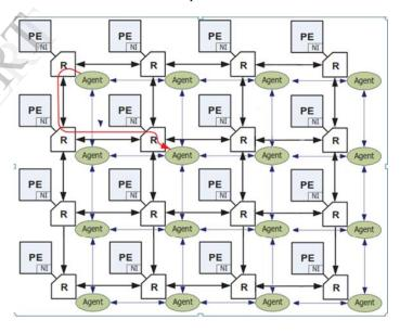
This 4x4 architecture is used in network to route the packets from one point to the destination point. Here the reliability is maintained to the best possible extent and the faulty units are completely avoided by information regarding the neighboring unit status.
