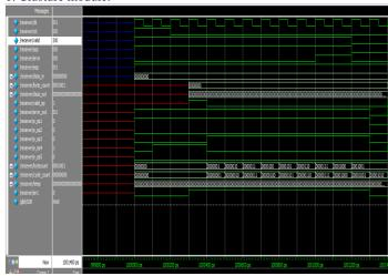
The result can be seen for various values of Data\_in for the respective selection of VALID, LDA, ERROR and RST respectively.
