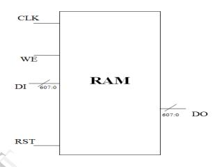
Features of RAM: WE pin is used to select the RAM in read=0 or in write=1 mode.DI is a data-input pin and DO is the data output pin respectively with 76bytes of capacity.Whenever the reset is high the DI and DO operation is halted.Clk has speed ranging from 4 MHz to 25 MHz's.
