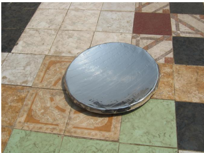
Fig. 2.5. Final dish after application of solar reflective film
