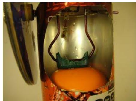
Fig. 2.4. Final assembly of prototype Stirling engine model
