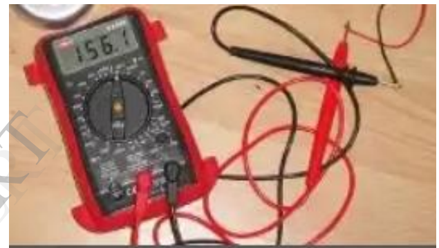
Fig. 5.3. Image depicting voltage reading 156 mV
