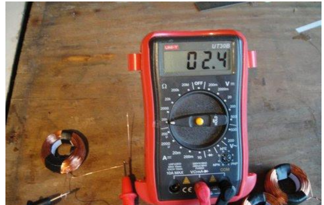
Fig. 5.2. Image depicting resistance reading 2.4Ω
