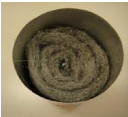
Fig. 2.1. Steel wool displacer inside a can serving as a pressure vessel
