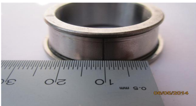
Figure 3.2: Photograph of inner race of taper roller bearing having groove defect width of 0.5 mm generated by EDM process
