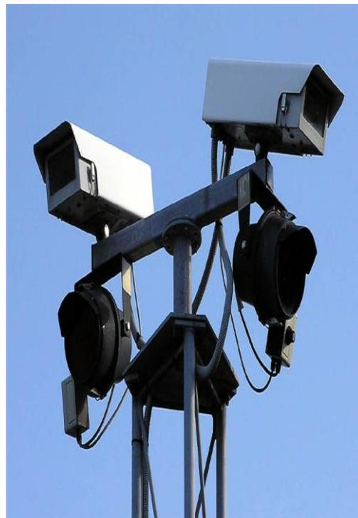
Figure 1 Closed-circuit camera [3] such as these can be used to take the images scanned by automatic number plate recognition systems.
