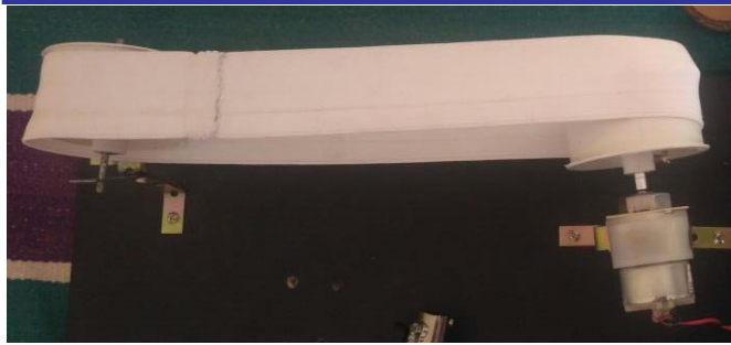
Fig. 4. Conveyor belt system
