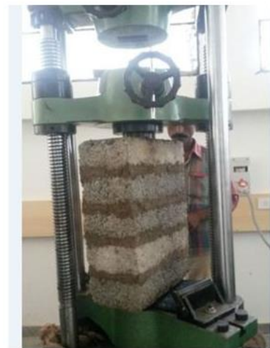
Fig.2.3: Testing of Masonry Prism
