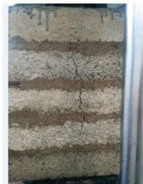
Fig.2.4: Crack Pattern of Masonry Prism
