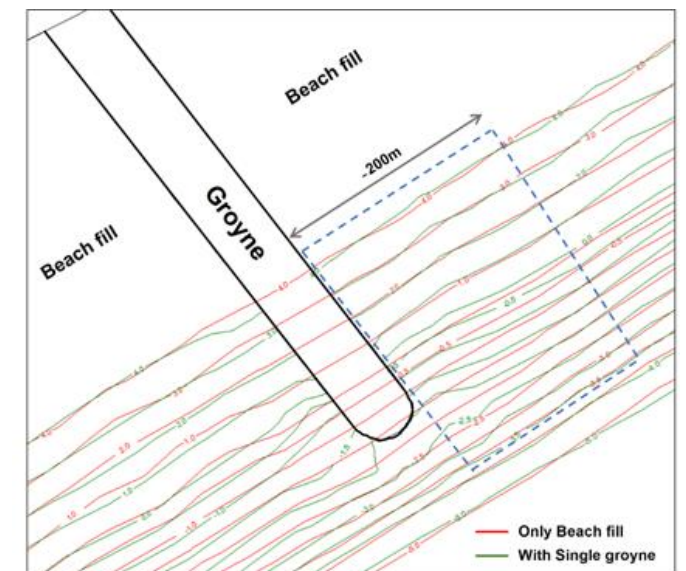
Fig. 3. Final Bed Level in Downdrift Portion of Groyne
