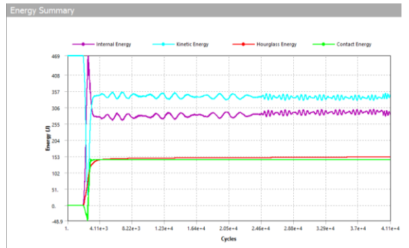
Fig 14.22 mm thickness Energy absorption
