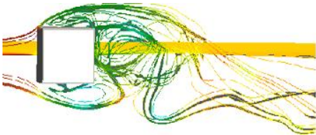
Fig 46. Horse shoe vortex at the backward face of the cube
