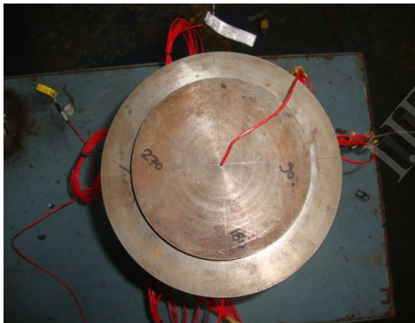
Figure 3: Location of thermocouples at different location on fins surface
