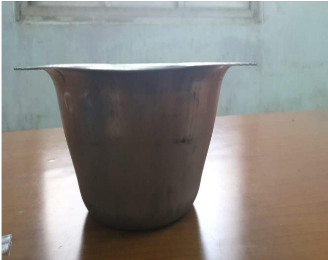
Fig. 10.. Semi-finished product with thickness 0.85mm (with draw bead)
