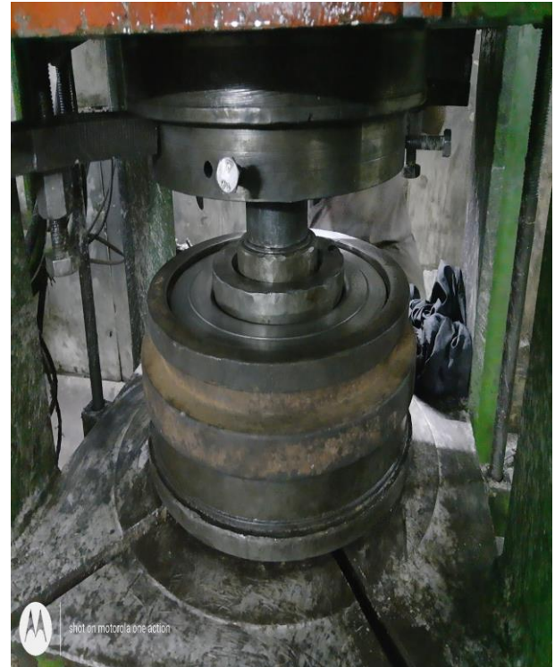
Fig. 8. Practical draw die setup without draw bead
