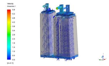
It can be seen from the flow chart that the flow field area in the whole carbon tank is mainly concentrated in the adsorption port and atmospheric port area with high velocity, and the flow velocity in other positions of the flow field is not high, and the flow velocity in the carbon powder area is below 0.5m/s.
