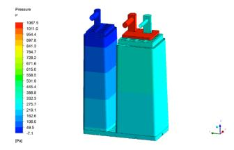
It can be seen from the three-dimensional pressure distribution diagram of the carbon tank that there is a significant pressure distribution at the atmospheric opening and adsorption opening, and the pressure range of the atmospheric opening is about -7.1 -- 49.5p, and the pressure at the adsorption opening is the largest, about 1000P. The pressure distribution in the flow field area of the carbon tank is uniform and has obvious pressure gradient.
