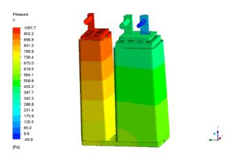
It can be seen from the three-dimensional pressure distribution diagram that the atmospheric opening and the desorption opening have obvious pressure distribution, and the pressure at the atmospheric opening is the largest, about 1000P,
