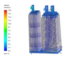
It can be seen from the flow chart that the flow field area in the whole carbon tank is mainly concentrated in the area of desorption port and atmospheric port with high velocity, while the flow velocity in other positions of the flow field is not high, and the flow velocity in the carbon powder area is below 1.2m/s.
