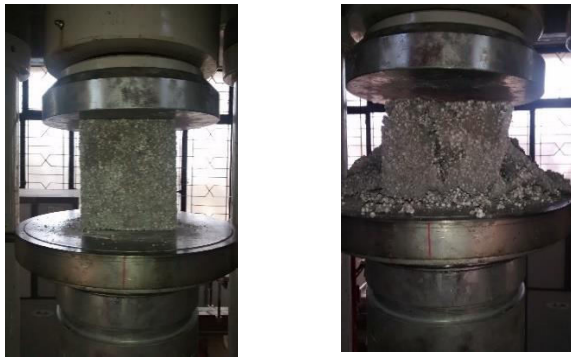
3a. Cube under compression 3b. Failure pattern Fig.3 Compression test on cubes
