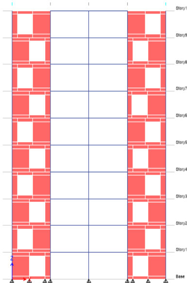
Fig 2: Elevation of the Frame-Shear Wall Building with Staggered Openings
