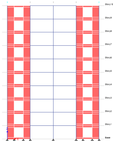
Fig1: Elevation of the Frame Shear Wall Building With Vertical Openings
