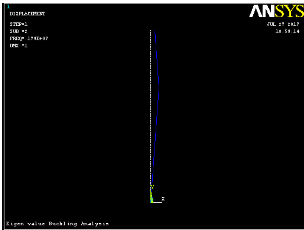
Fig.4: Buckling mode (2) - Model (1)
