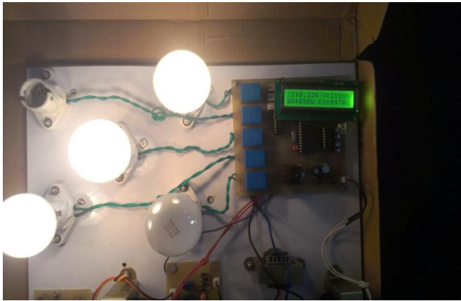
Fig 2. Switching off of the least priority load
