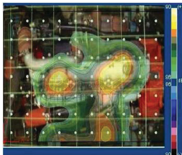
Figure 4.2.1 Noise Grid Method [3]
