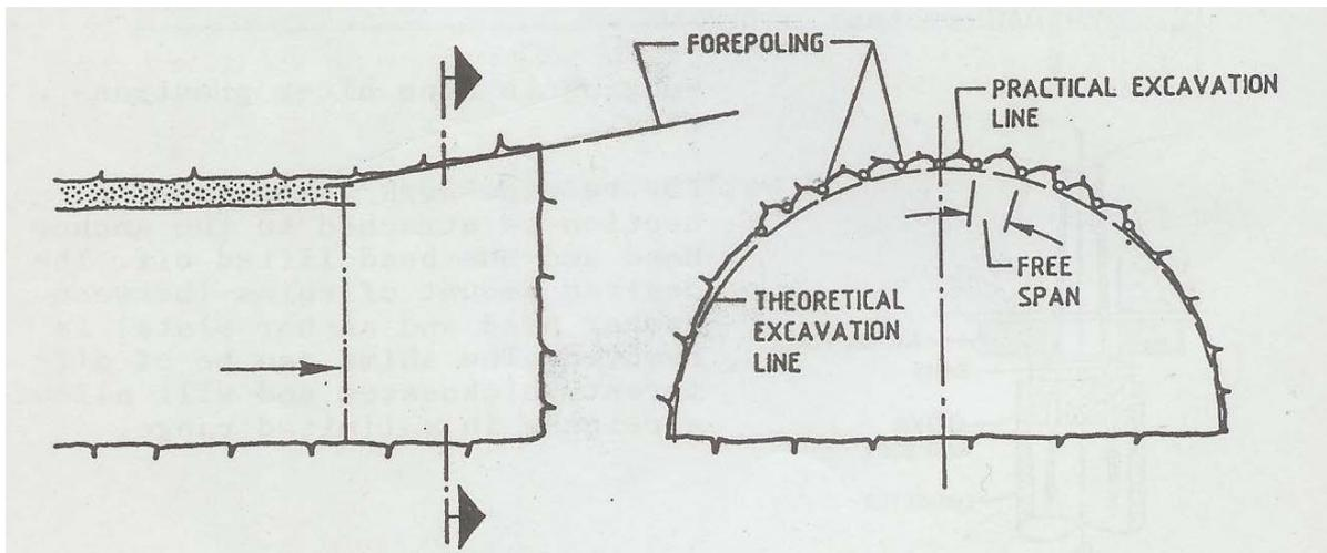
Fig.25 Construction Steps:
