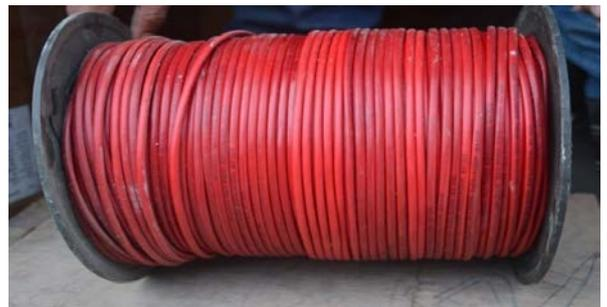
Fig. 6 Detonating cord/cortex
