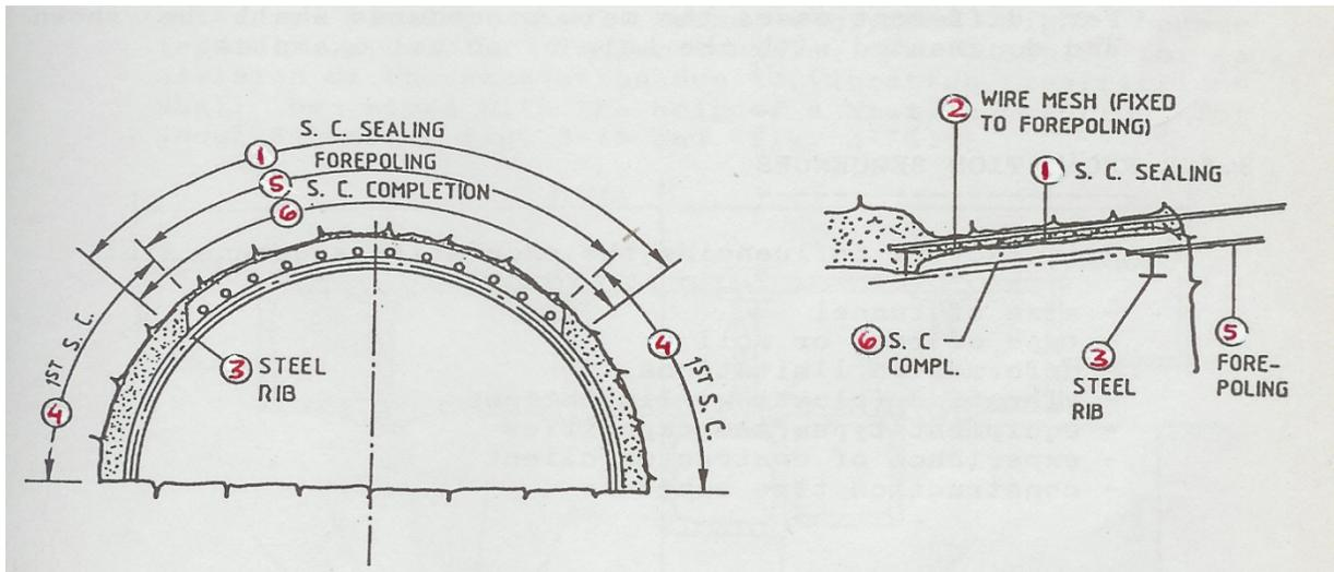
Fig. 24 Shape of Excavation with Forepoling
