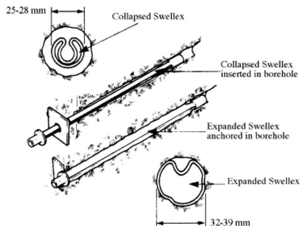
Fig. 34 Swllex Rock Bolt
