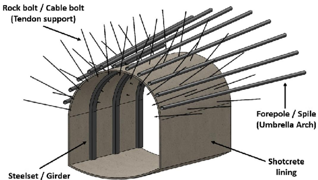
Fig. 29 Tunnel Profile with rock bolts and forepoles
