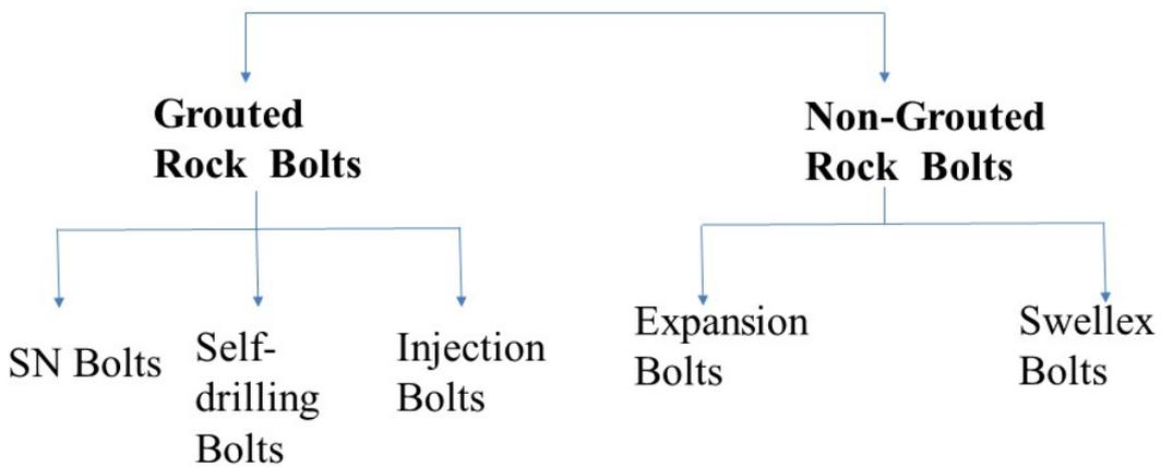
Fig. 28 Flow Chart of Types of Rock Bolts
