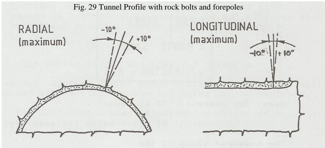
Fig. 27 General the Direction of Rock Bolts
