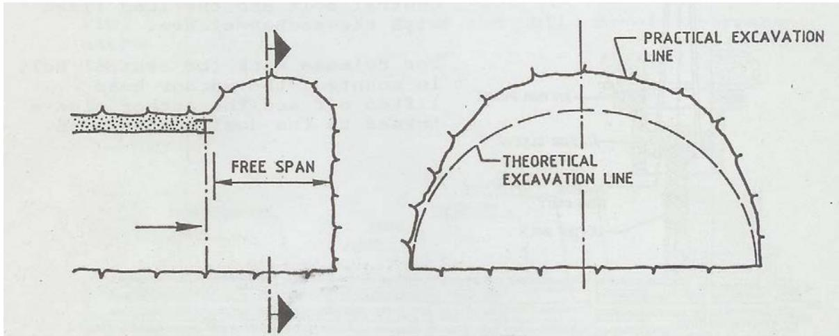
Fig. 23 Shape of Excavation without Forepoling
