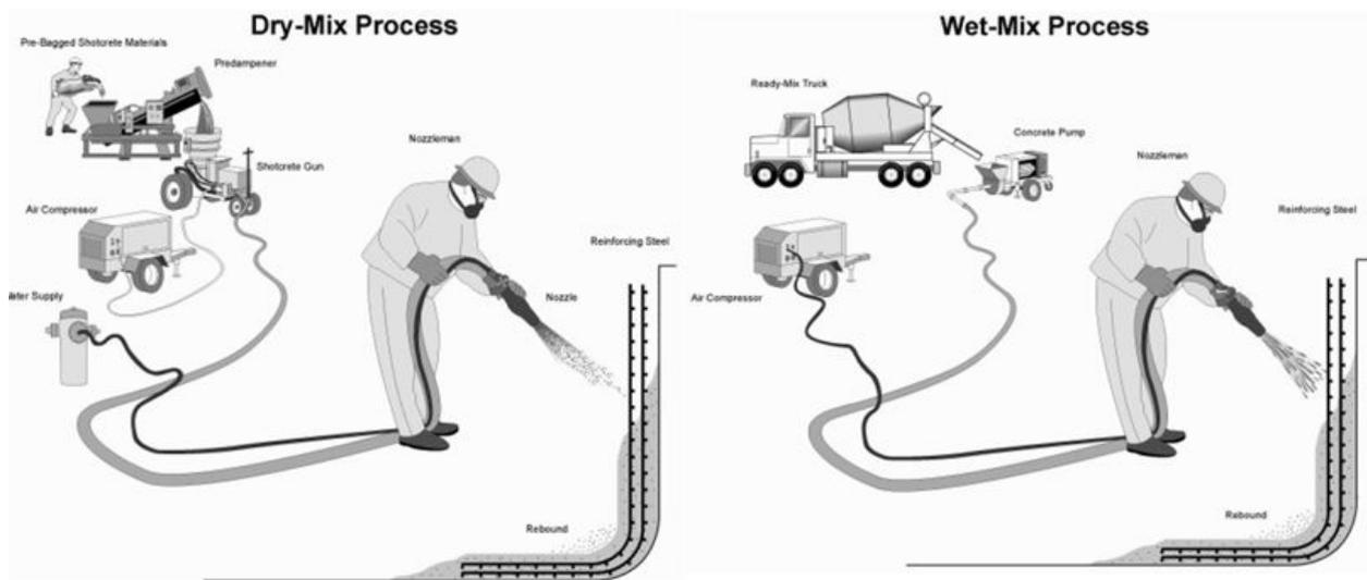
Fig. 26 Shotcrete methods : (a) Dry method; (b) Wet Method
