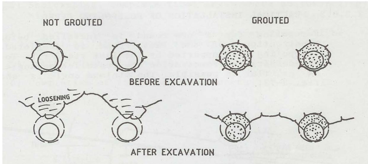
Fig. 35 Difference between not grouted and grouted forepoling installed in pre-drilled holes
